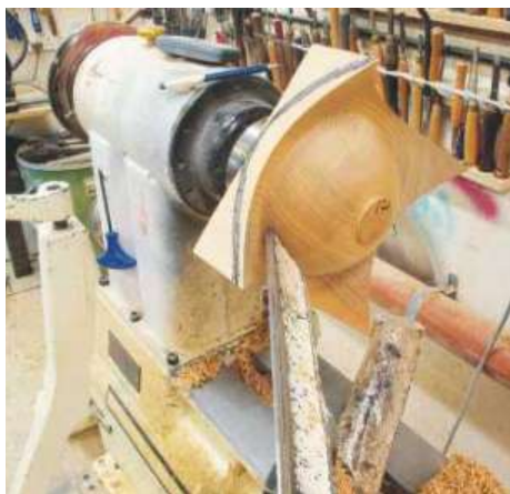
▲ Pic.13 I have managed to get the toolrest inside the wings, but the problem with this is that I'm going to be working right on the end of the blank. Make sure everything is tight here as if it moves, you'll break the piece
